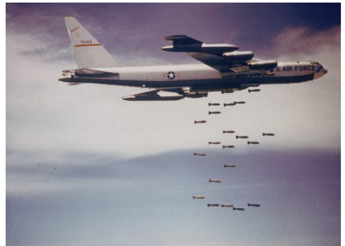
A B-52 bomber drops bombs over North Vietnam. The B-52 was designed to carry nuclear bombs. It could carry up to 70,000 pounds of bombs.
